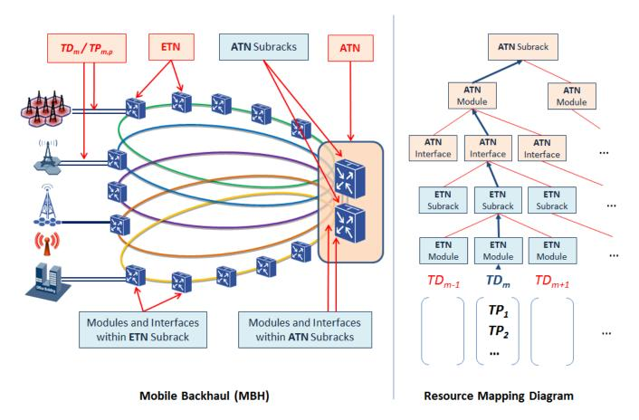
Fig. 2: MBH resource assignment and mapping diagram  $TD_m$ : Traffic Demand for ETN Module m,  $TP_{m,p}$ : Traffic Profile p activated in module m
