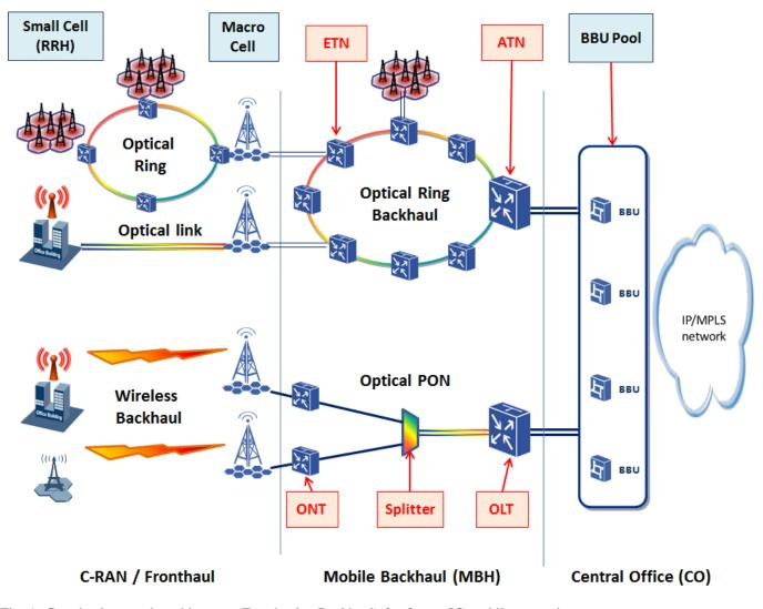
Fig. 1: Crosshaul network architecture (Fronthaul + Backhaul) for future 5G mobile networks. ETN : Edge Transport Node, ATN : Aggregation Transport Node
