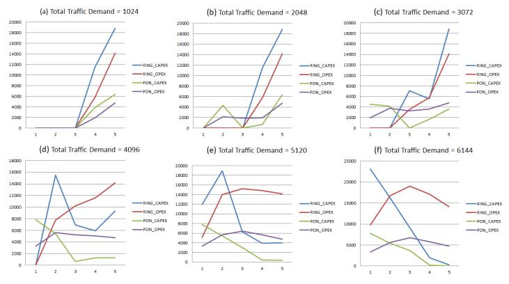
Fig. 6: CAPEX and OPEX yearly evolution for PON and Ring-based networks (using TPaaS)
